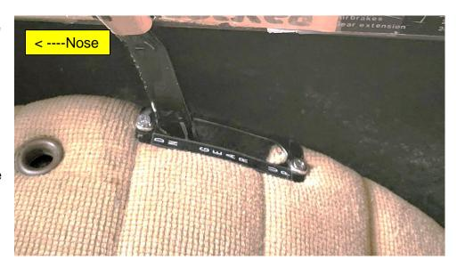
position was gear up and which was gear down on the Grob 102 and even some with solid knowledge of and experience flying the aircraft got it wrong.) Here's the label.
