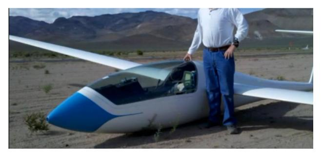
If you touch down and realize that you forgot to put the gear down, just ride it out. Attempting to lift the aircraft back in the air, swapping control stick hands, putting the gear down, swapping hands again, and touching down again could end badly.
