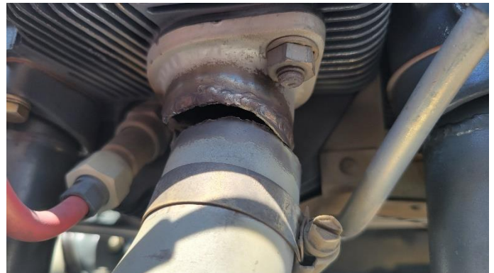
Broken Exhaust Pipe
