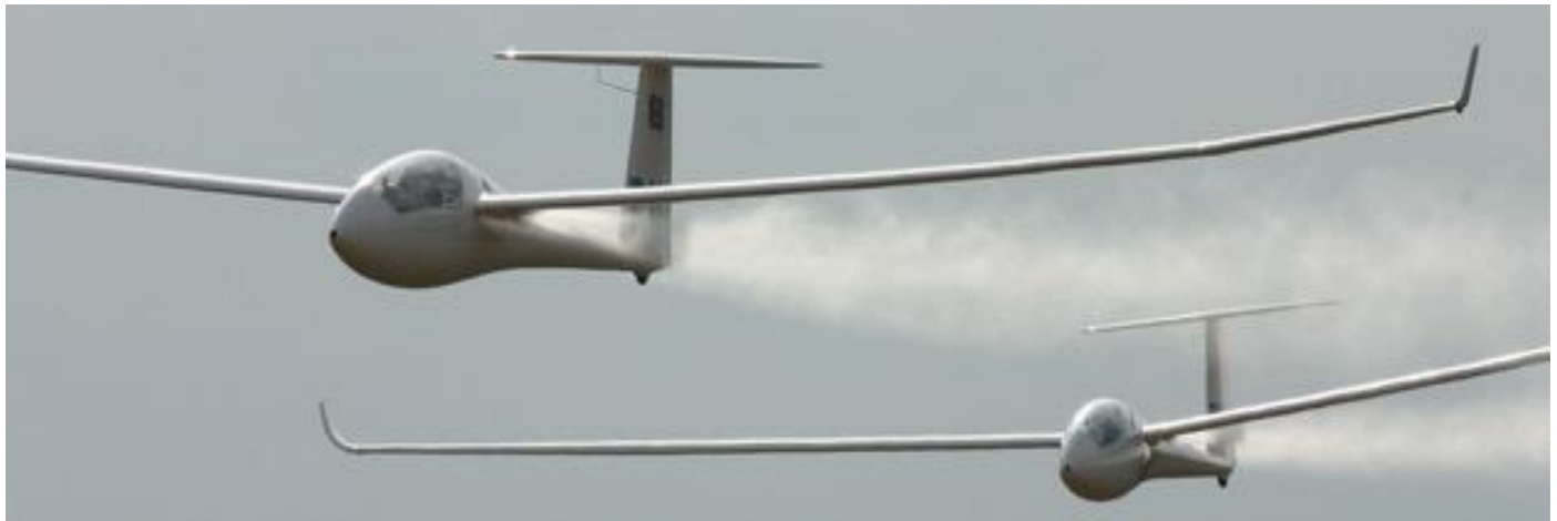
Gliders finishing a race photo by astir698. The vapor you see is from the dumping of water ballast. Gliders load up with water before they launch and get rid of the extra weight before they land. A heavier glider will fly faster, increasing distance and speed points for the flight.
