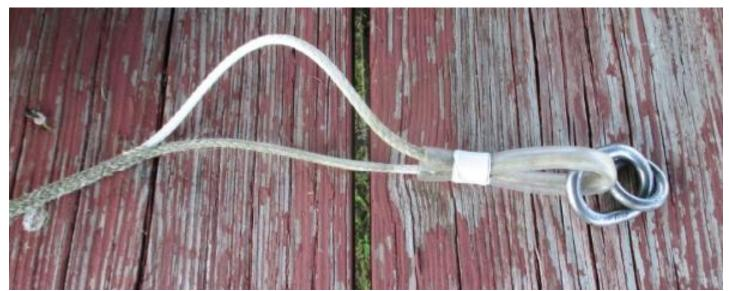
When preparing to launch a subsequent flight, it was discovered that the inner line had come completely out of the outer on the glider end of the tow rope itself.
