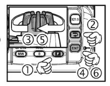
**NOTE:** You can override/disable the squelch by depressing the Monitor button on the left side of the radio for 2 seconds. Squelch is re-enabled by momentarily pressing the Monitor button.
