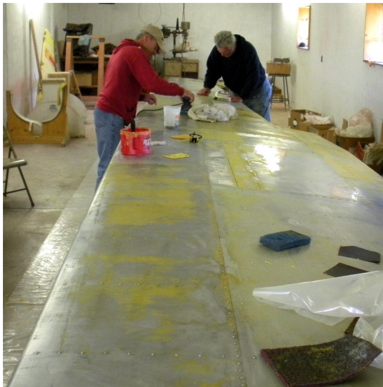
Mark Miller and Ron Kellerman removed paint from the wings of N3616Q. Photo: JCD
