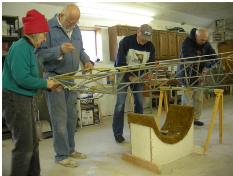
Wednesday Crew removing light rust from tubing.
