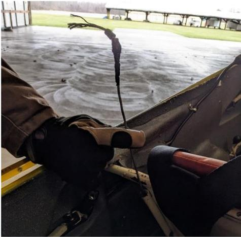
15H is now red-tagged, because the cable securing the canopy broke on landing (see picture).
