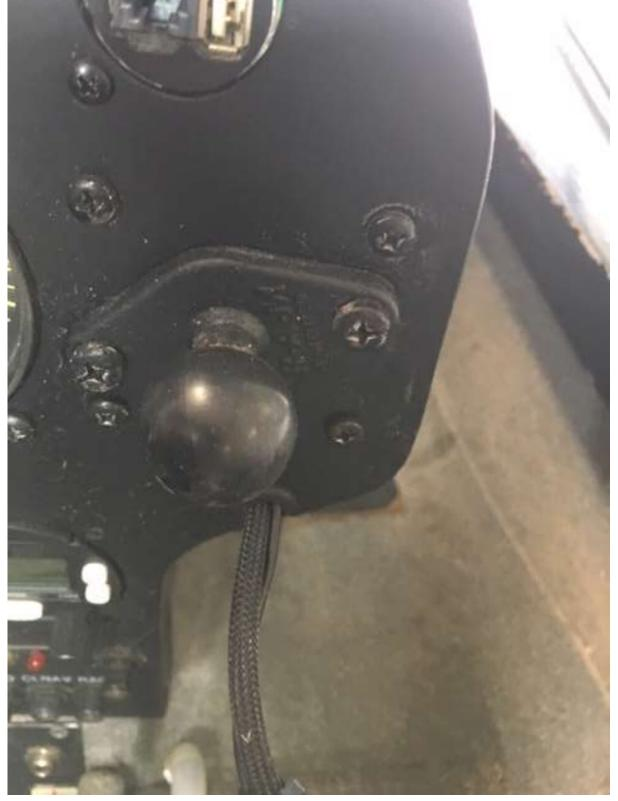
Dick Huskey recently installed a 1inch Ram Mount to the front instrument panels in all the CCSC gliders (Thanks Dick).
