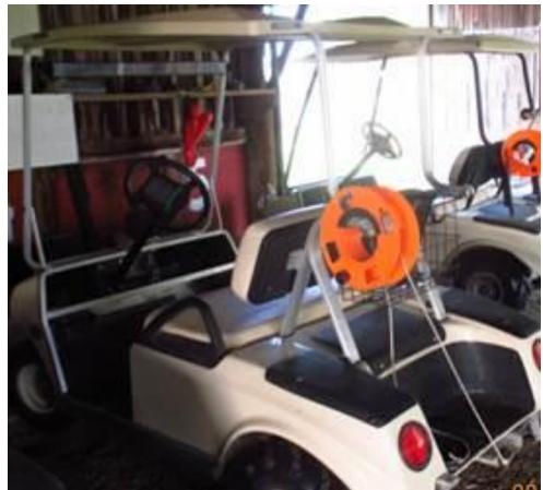
wheels he and Keith Kilpatrick designed, built and installed on the golf carts. There is a loop tied in the rope at the midpoint. This loop is placed over a hook inside the take-up wheel and then wound up quickly, keeping the rope neatly stowed until next use. I am looking forward to using them!
