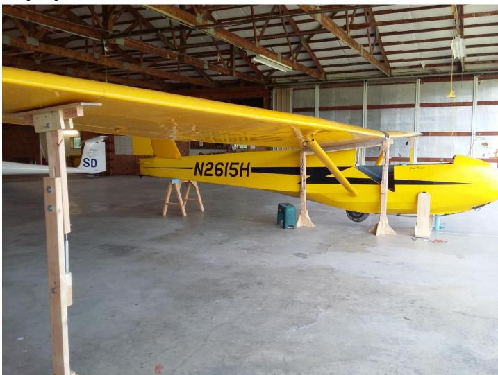
Special thanks to Steve Statkus and Keith Kilpatrick for their design and construction of custom assembly stands and special wing root allignment tools for installing (and removing) 2-33 wings and struts. In the past it took a team of about 6 or more to struggle, twist, force, beat and curse over several hours; now 3 guys can simply lift the wings into place and insert the locking bolts. GREAT JOB!
