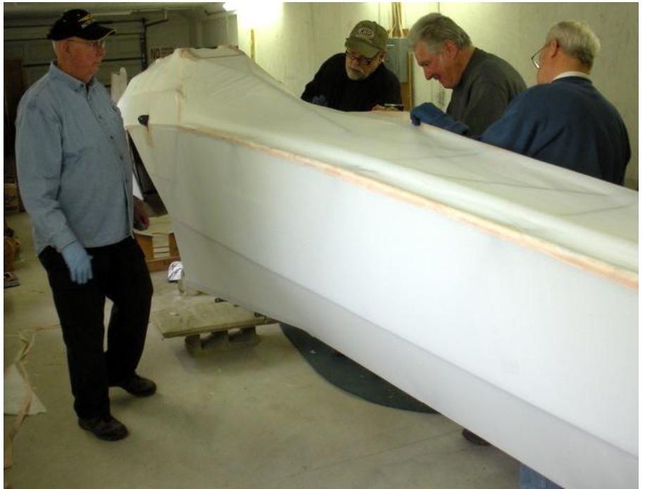
(l. to r.) Lynn Alexander, Steve Statkus, Ron Kellerman and Bill Hall glue the final big sheet of fabric into place on the aft lower surface on Wednesday.
