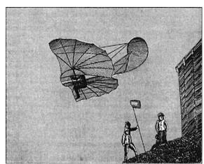
Between 1866 and 1889 German Otto Lilienthal tested numerous cambered surfaces with a Caley-like (see last month's article) rotating-arm testing device that measured up to 23 feet long. His studies of wing camber and the resulting lift were flawed, however, leading him to believe that powered flight would be forever impossible.
