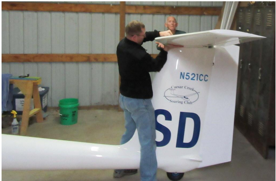
John Dudley and Dick Scheper prepare to remove the horizontal stabilizer. Photo: Jim Dudley
