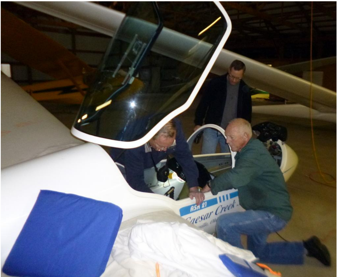
After the front canopy was removed the seat cushions and seat panels were removed. Photo: Norm Leet
