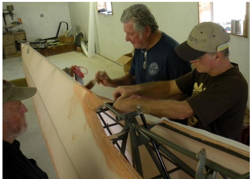
Tom Bonser (l) monitors progress as Ron Kellerman (c) and Keith Kilpatrick (r) apply reinforcing tape to a glue joint.
