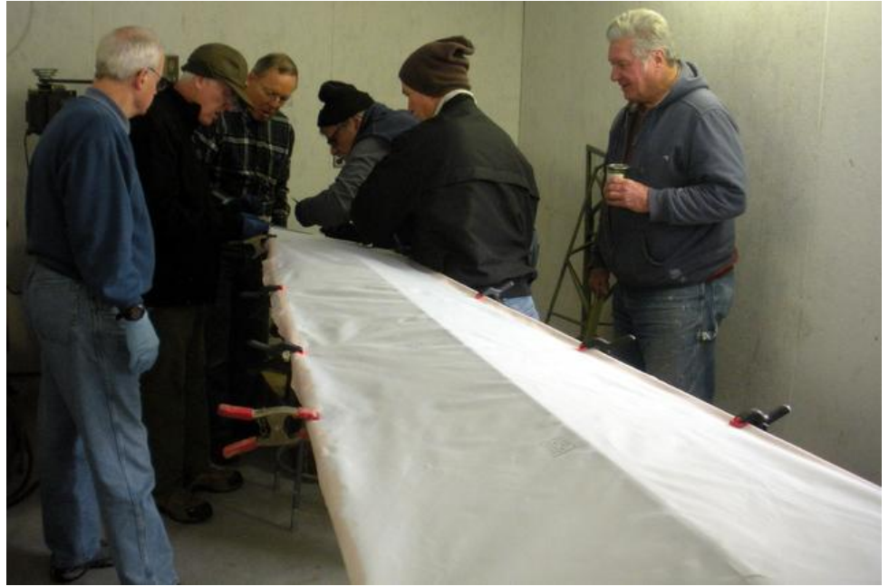
The crew commenced gluing fabric to 16Q's fuselage on Wednesday and continued on Saturday.
