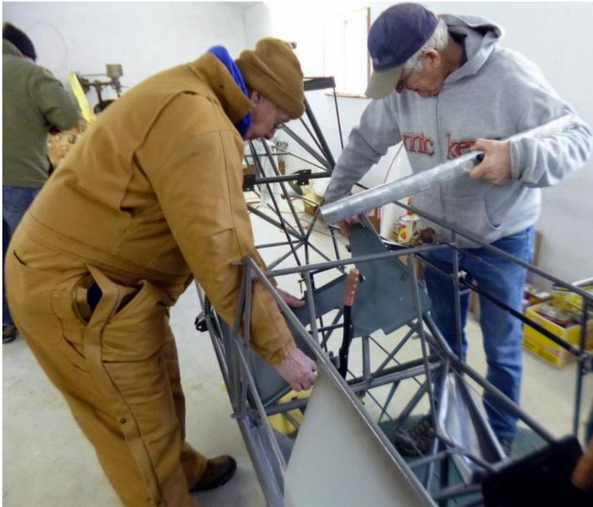
**Lynn Alexander and Dan Reagan check the fit of the new interior panels that Dan has fabricated. The frame has been moved to Dan's hangar/shop to facilitate fitting the new panels.**
