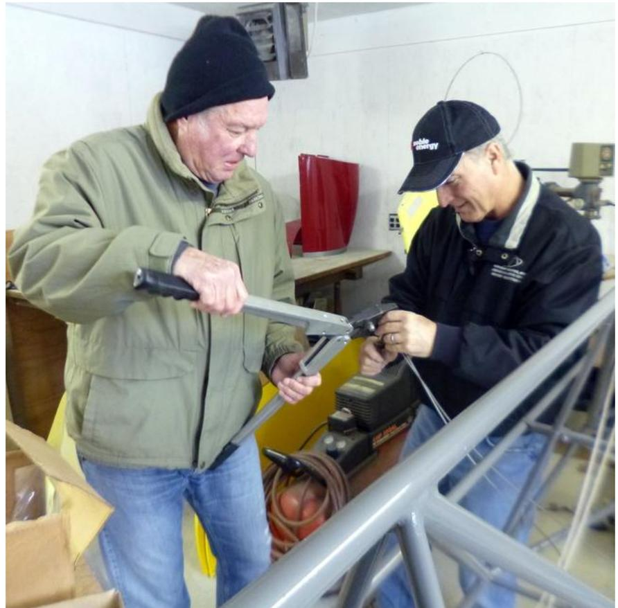
**After the new cables had been treaded into place and length verified, the loops at the ends were crimped in place by Ron Kellerman and Keith Kilpatrick.**
