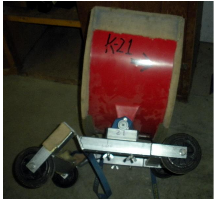
Trailer dolly with K21 cradle. A similar cradle for the G103 can be installed on the same dolly. Be sure you use the right one.
