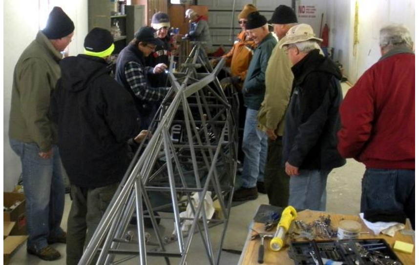
Early Wednesday we continued assembling the control components onto the frame and made control cables.
