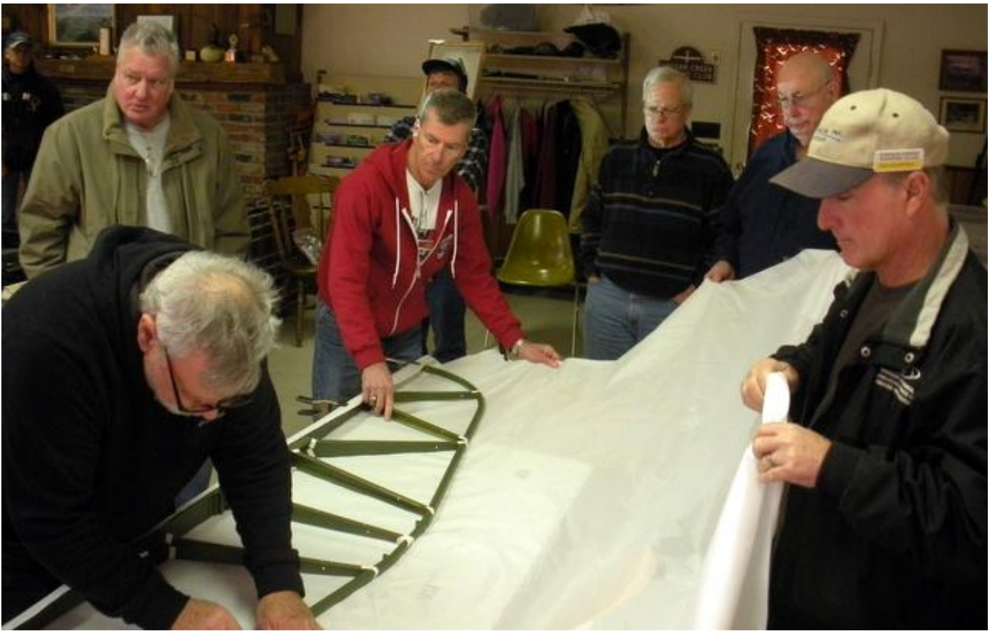
Fabric is marked for cutting for one surface of Lynn Alexander's horizontal stabilizer.
