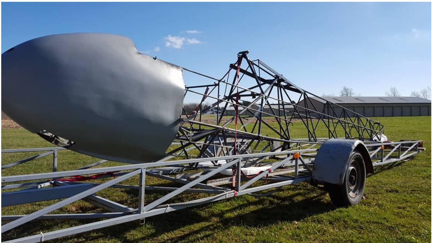
Freshly painted frame for 16Q returned to CCSC on Saturday. Reassembly of interior components will take place Wednesday.
