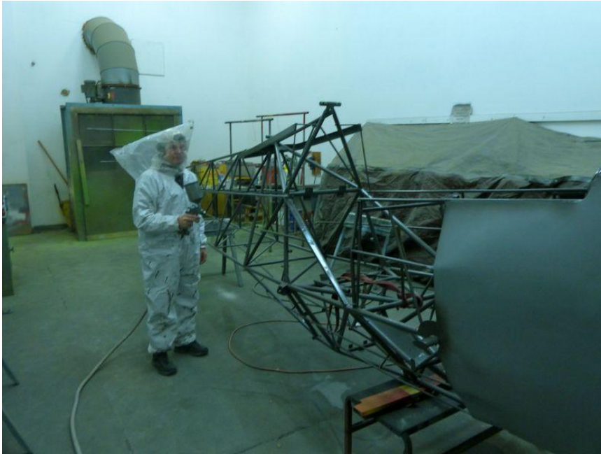
Tim Morris spraying grey epoxy paint onto frame of 16Q
