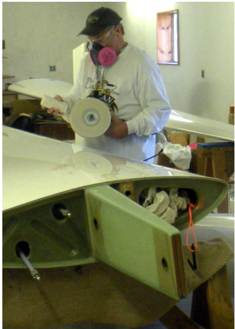
Here John Lubon is holding a bar of white wax in his right hand and pressing it against the rapidly rotating cloth buffing wheel on the heavy duty grinder motor in his left hand.
