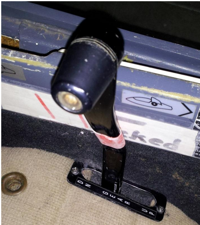
Handle at GEAR - Down but NOT LOCKED
