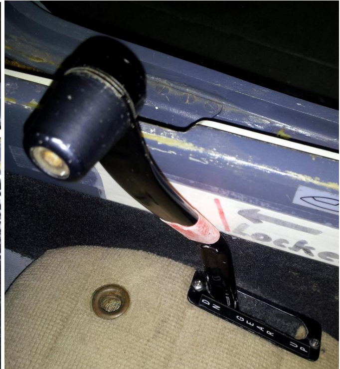
Handle at DN - Gear down and LOCKED
