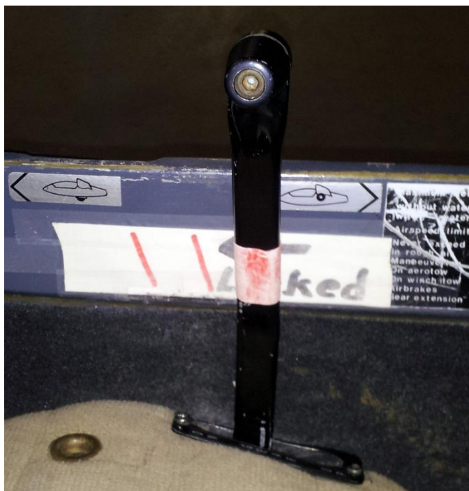
Landing gear down but NOT LOCKED
