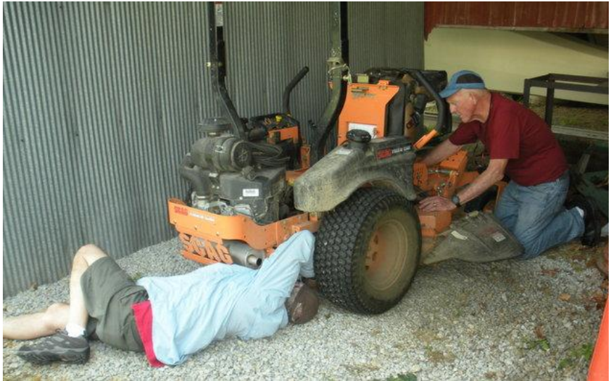
Dan Reagan and Dick Scheper installed a new belt on the Skag mower on Wednesday. On Sunday Jim Marks finished the project, installing three new blades.
