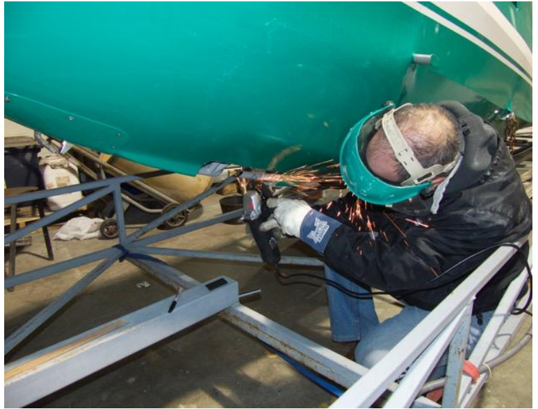
New Member, Keith Kilpatrick, removing bent keel tube.
