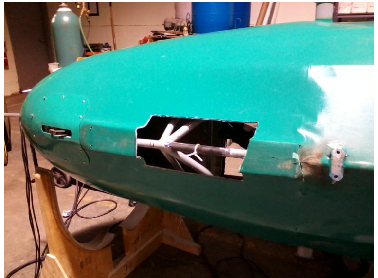
New section of keel tube with internal doubler installed.
