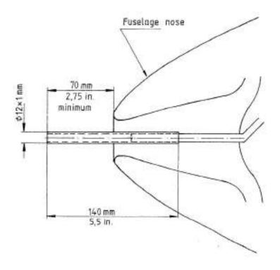
Brass tube 5,5 in = 140 mm in length (12 0 x 1). One may also use a suitable plastic tube provided that it is sufficiently stiff and straight.
